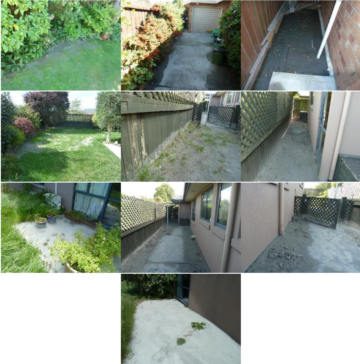
Figure 47: Ground photographs of ejecta on the properties in the NE quadrant of the 50-m buffer (photograph date: Nov 2011).
